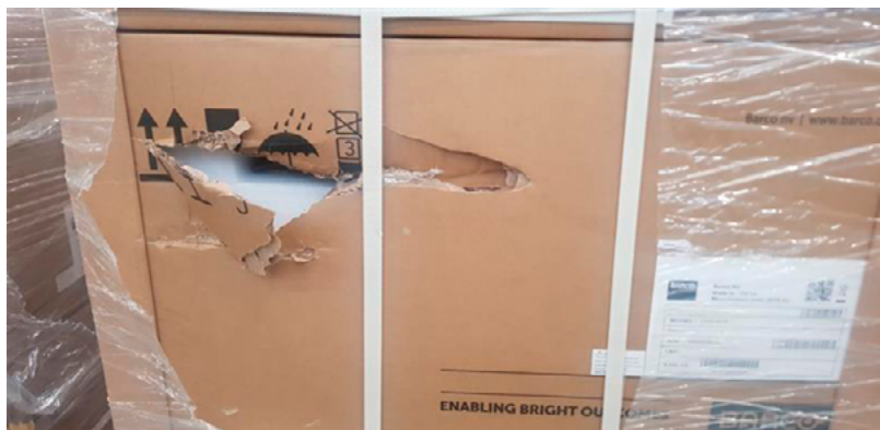
Figure 29. Damage on the exterior of a transport package
