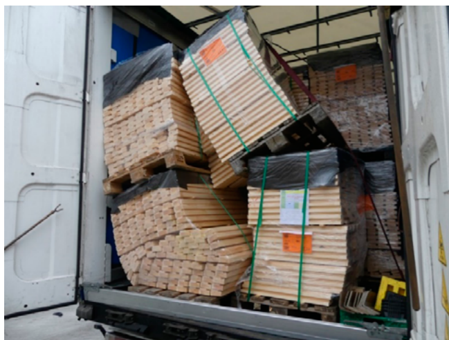
Figure 30. Insufficiently lashed and secured wood material load in a CTU
