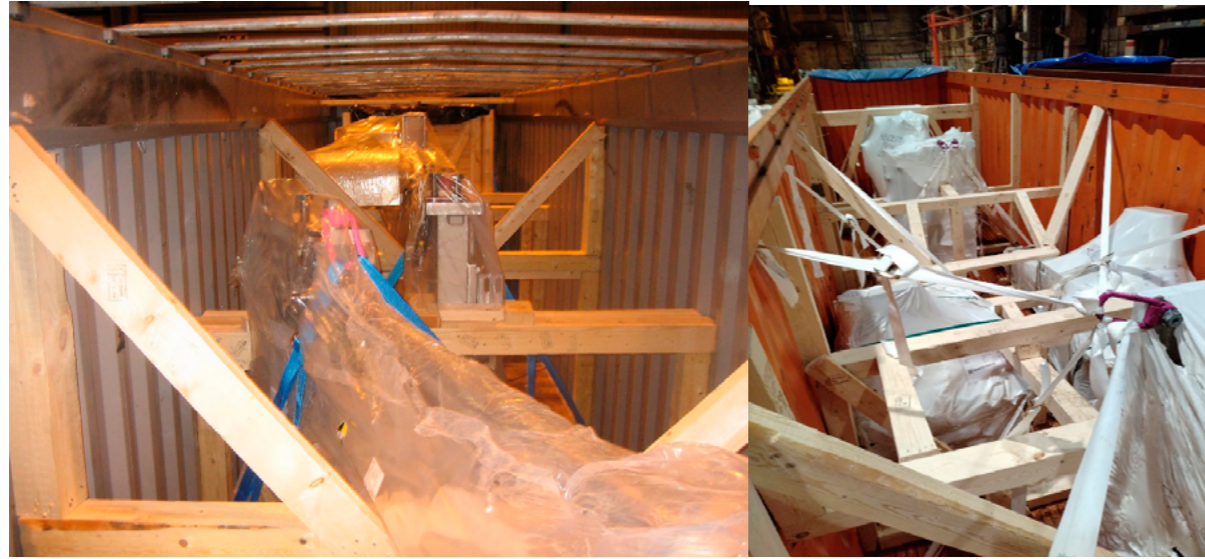
Figure 64. Example images of blocking inside of a CTU Photo: Valmet Technologies, Inc.
