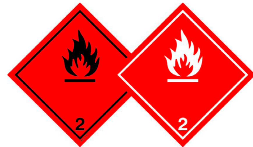
Figure 60. Illustration of warning labels (Storck Guide, Stowage & Segregation to IMDG Code 2023)
