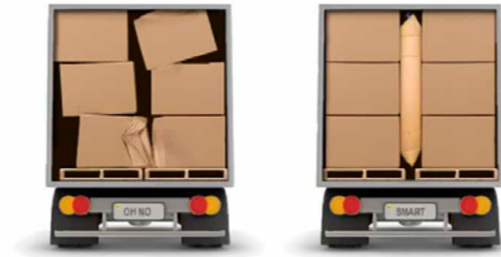
Figure 41. Supporting light cargo parcels with dunnage bags: unsupported cargo on the left side, cargo supported with a dunnage bag on the right side
