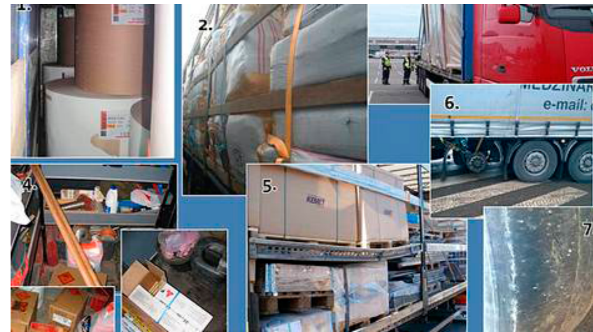
Figure 31. Examples of inadequate cargo securing. Photo: Helsinki Police Department/Iltasanomat (2015). https://www.is.fi/autot/art-2000000964731.html
